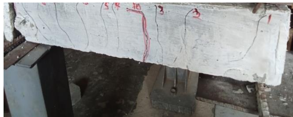
Plate 8: Flexural Test Set-up Plate 9: Cracks on High Strength Reinforced Concrete Beam Sample
