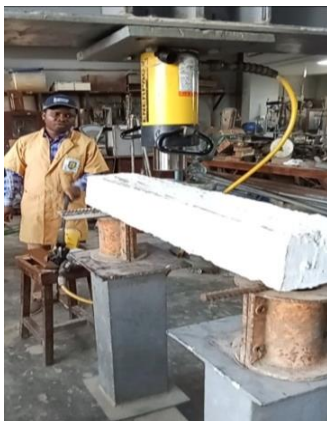
Plate 8: Flexural Test Set-up Plate 9: Cracks on High Strength Reinforced Concrete Beam Sample
