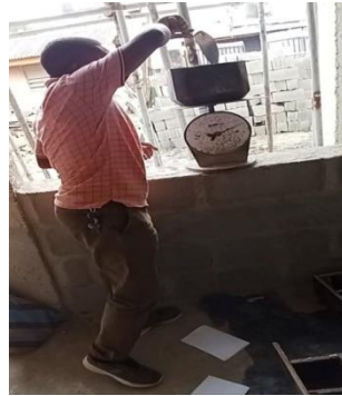
Plate 5: Weighing of Concrete Materials
