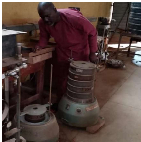
Figure 2: Mechanical Sieving of Materials
