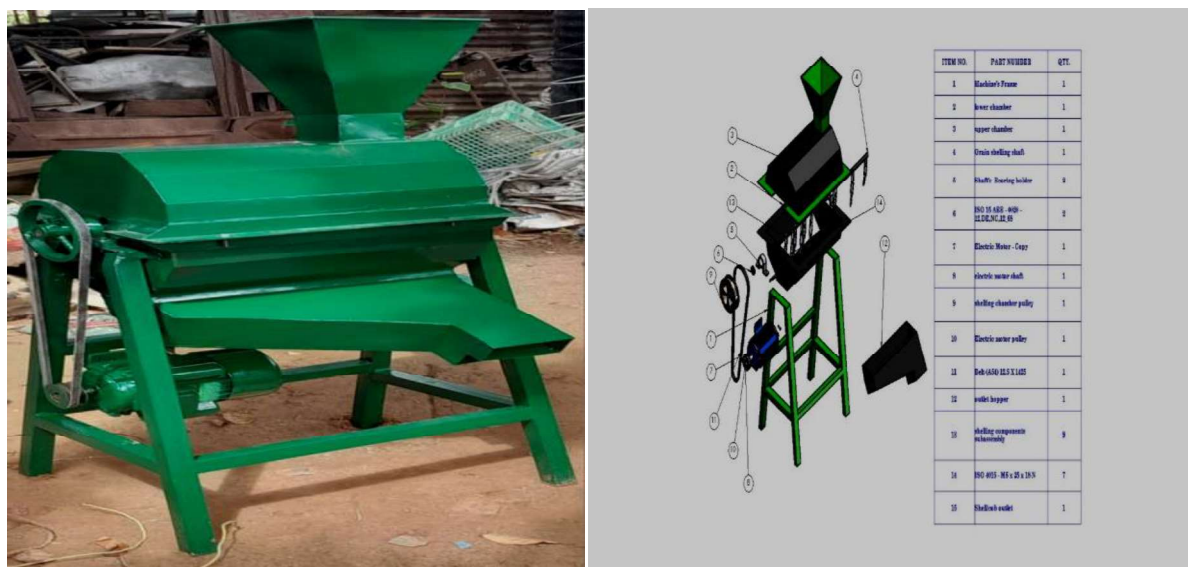
Fig 1: Assembly Drawing Showing the Various Components of The Multi-Variant Shelling Machine.
