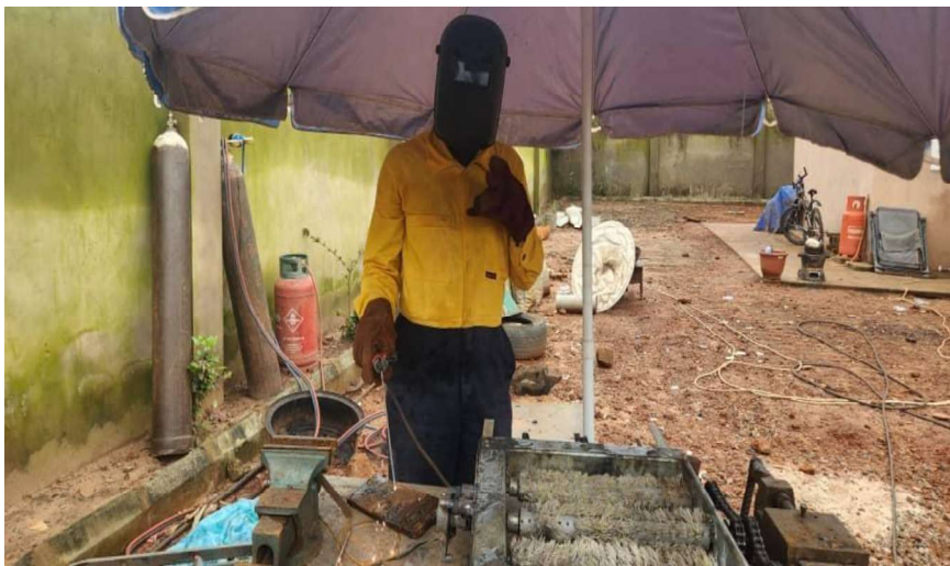
Fig 1: Welding of the sprocket
