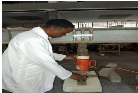
Plate 5: Marking off support and load path as guided by ASTM 293C code
