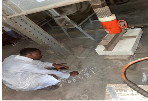
Plate 8: Reading out values of ultimate load and deflection from dial gauge
