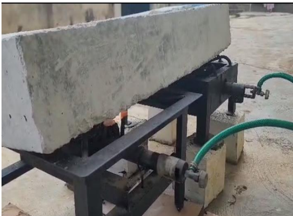
Plate 3: Concrete beam heated to 600°C
