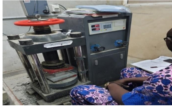
Plate 2: Compressive test of concrete cubes
