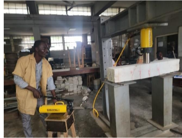
Plate 5: Beam sample under flexural testing
