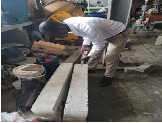
Plate 4: Rebound hammer test on beam
