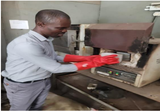
Plate 1: Heating of concrete cubes
