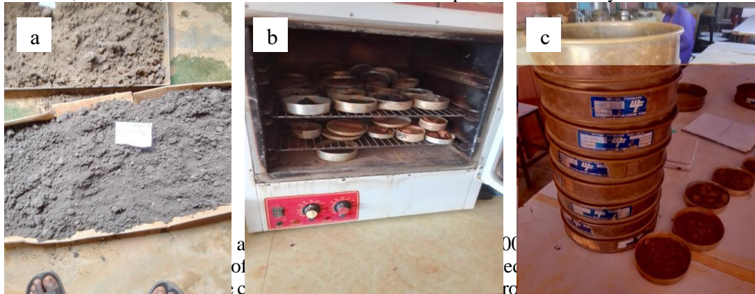
B Figure 2: View of a) soil sample b) moisture content test c) sieve analysis according to BS 1377-4:1970 standards.
